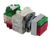
Push button, Harmony 9001K, 30mm 2 push buttons, with pilot light, green marked START / red ON / red marked STOP, 10A, 600V AC, 1NO + 1NC
