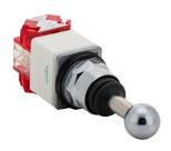
Joystick controller, Harmony 9001K, metal, 30mm, 2 directions, spring return to center, 2NO
