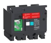
Earth-leakage add-on protection module VigiPacT, ComPacT NSX 100/160, 200VAC to 440VAC, 30mA to 30A, 3 poles
