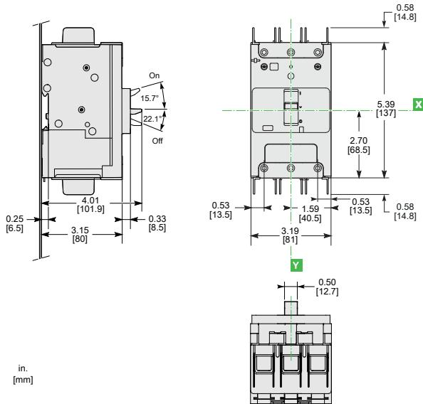
(F) TERMINATION OPTION - Terminal Nut (ON end) / Terminal Nut (OFF end)
