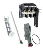
Operating mechanism, flange mounted, variable depth, 60A, 600V, no fuse, switch mechanism, 6 inch handle, NEMA 4
