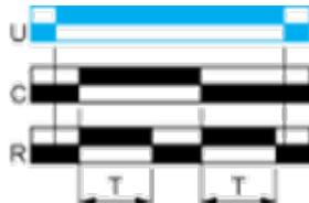
**Function C : Off-Delay Relay with Control Signal**
