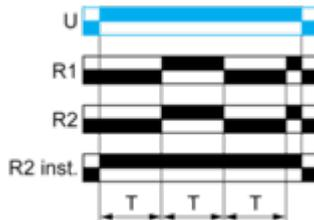
**Function: 1 Output with Retrigger / Restart Control**
