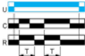
**Function Bw : Double Interval Relay with Control Signal****Description**
