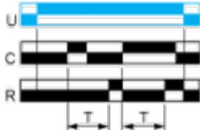
Function Ah : Pulse Delayed Relay (Single Cycle) with Control Signal**Description**
