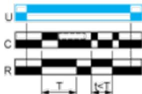
**Function W : Interval Relay with Control Signal Off**
