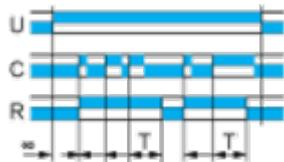
**Function O : Retriggerable Interval Delayed Relay with Control Signal On**
