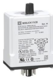
Timing Relay, Type JCK, plug In, on delay, adjustable time, 0.1 to 10 seconds, 10A, 240 VAC, 120 VAC/110 VDC
