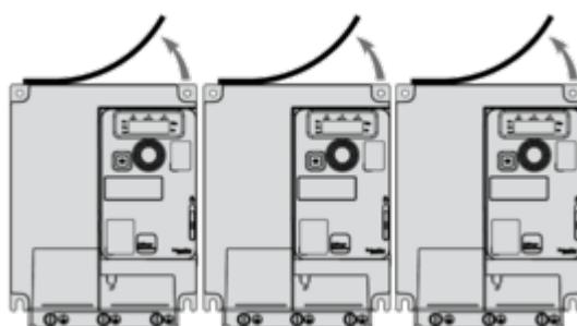
**Mounting Type C: Individual, Ventilation Cover Removed**
