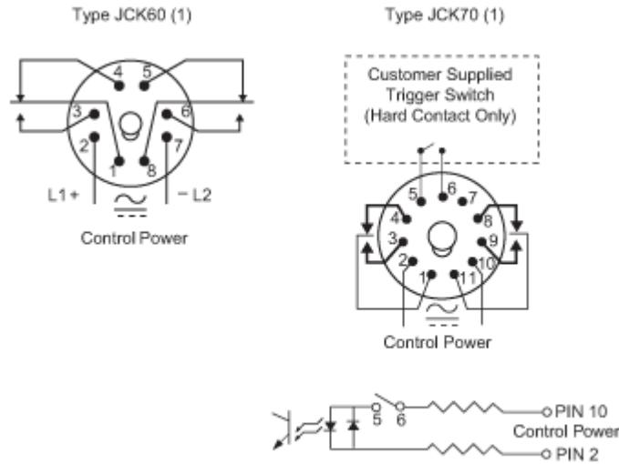
(1) Do not apply DC voltage to the 240 Vac timers (voltage code V24).
