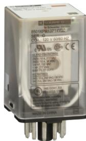
Plug in relay, Type KP, tubular, 1 HP at 277 VAC, 10A resistive at 120 VAC, 11 pin, 3PDT, 3 NO, 3 NC, 120 VAC coil
