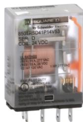
Plug in relay, Type R, miniature, 1 HP at 277 VAC, 15A resistive at 120 VAC, 5 blade, SPDT, 1 NO, 1 NC, 24 VDC coil
