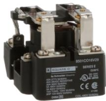
**Power Relay, Type C, 2 hp, 30A resistive at 300VAC, DPDT, 2 normally open and 2 normally closed contact, 480VAC coil**
