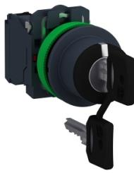
Selector switch, Harmony XB5, flush mounted sw. key 455 3 pos stay put key release 3 pos 2 NO screw
