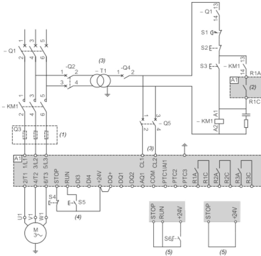
(1) : Installation of additional fast-acting fuses to upgrade to type 2 coordination according to IEC 60947-4-2.
