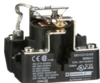
**Power Relay, Type C, 2 HP, 30A resistive at 300 VAC, SPDT, 1 normally open and 1 normally closed contact, 120 VAC coil**
