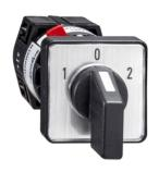
Complete cam switch, Harmony K1, K2, cam changeover switch, 16mm or 22mm, plastic, 3 poles, position 0, 60degrees, 10A, 30x30mm, marked 1 0 2
