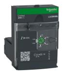
Advanced control unit, TeSys Ultra, 3P, 1.25 to 5A, 690VAC, protection & diagnostic, class 10, 24VDC coil
