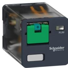
universal plug in relay, Harmony Electromechanical Relays, 10A, 3CO, without LED, lockable test button, cylindrical, 12V DC
