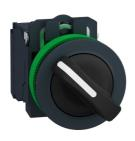
Selector switch flush mounted, Harmony XB5, plastic, black, 30mm, 2 positions, spring return right to left, 1 NO
