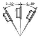
When installing this product in a slanted position with an incline more than 30°, the ambient temperature must not exceed 40 °C (104 °F). You may need to use forced air cooling (fan, A/C) to ensure the ambient operating temperature is 40 °C or less (104 °F or less).
