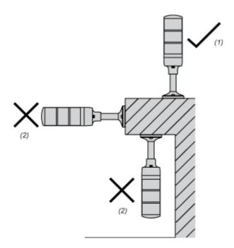
Choose a flat surface with enough strength and with little vibration for installation. Mount this product according to the figure to maintain IP characteristics.
