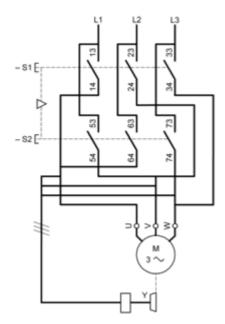
Control of Single-Speed Reversing Motor 3-Phase switching, Reversing by 2-Phase Inversion
