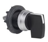
Cam switch operating head, Harmony K1, K2, mounting hole 22mm, plastic head with bezel 29mm, metallic legend, black handle
