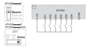
Switch Set to SRC (Source) Position and Use of an External Power Supply for the Digital Inputs
