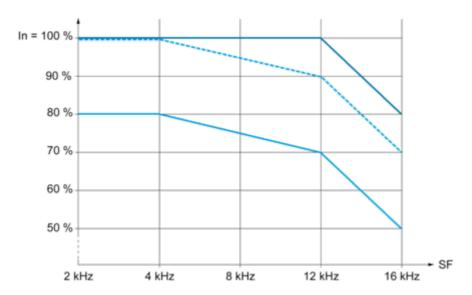
40 °C (104 °F) - Mounting type A, B and C 50 °C (122 °F) - Mounting type A, B and C 60 °C (140 °F) - Mounting type B and C
