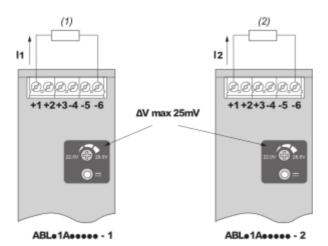
(1):  $R_{Load1}$ (2):  $R_{Load2}$  $R_{Load1} = R_{Load2}$  $I_1 = I_2 = \sim I_{nom}$
