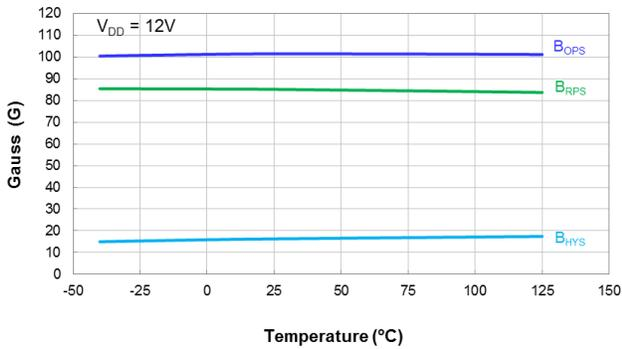
Switch Points B<sub>OPS</sub> and B<sub>RPS</sub> vs Temperature
