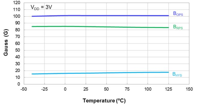
Switch Points B<sub>OPS</sub> and B<sub>RPS</sub> vs Temperature
