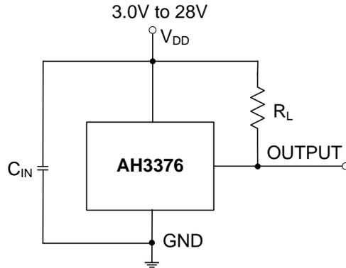
Note: 4.  $C_{IN}$  is for power stabilization and to strengthen the noise immunity, the recommended capacitance is 10nF ~ 100nF.
