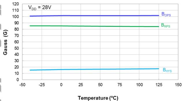
Switch Points B<sub>OPS</sub> and B<sub>RPS</sub> vs Temperature
