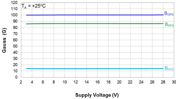
Switch Points B<sub>OPS</sub> and B<sub>RPS</sub> vs Supply Voltage
