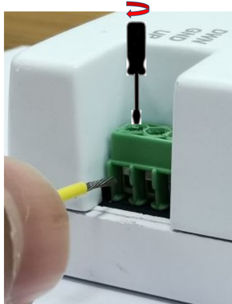
Figure 8 - Clamping wire with screwdriver in clockwise direction
