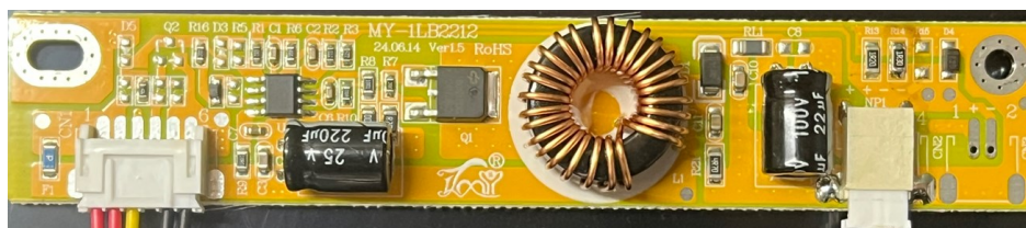
Figure 5 - LED Backlight Inverter Board Front View
