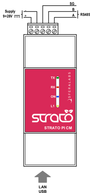
STRATO PI CM CONNECTION DIAGRAM
