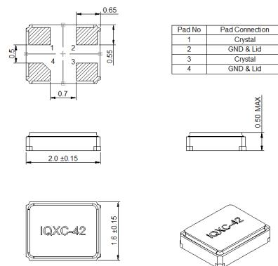
Note: The pad style on the base of the device may differ slightly from the drawing.
