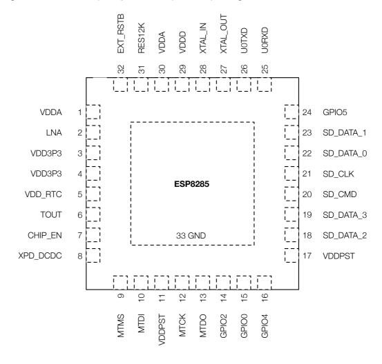
Figure 2-1. Pin Layout (Top View)
