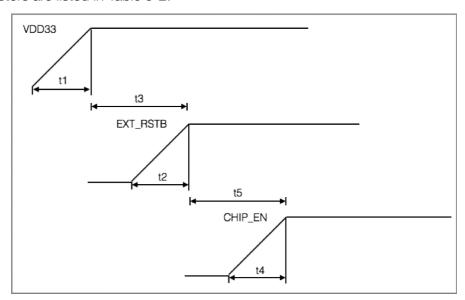
Figure 5-1. ESP8266EX Power-up and Reset Timing
