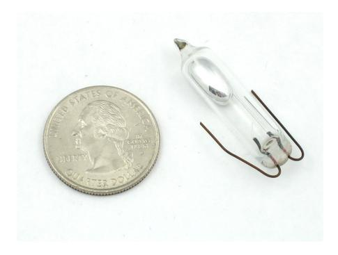
While not as precise or flexible as a full accelerometer, tilt switches can detect motion or orientation simply. Another benefit to them is that the big ones can switch power on their own. Accelerometers, on the other hand, output digital or analog voltage that must then be analyzed with extra circuitry.
