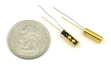
Tilt switches used to be made exclusively of mercury, but are rarer now since they are recognized as being extremely toxic. The benefits of mercury is that the blob is dense enough that it doesnt bounce and so the switch isnt susceptible to vibrations. On the other hand, ball-type sensors are easy to make, wont shatter, and pose no risk of pollution.
