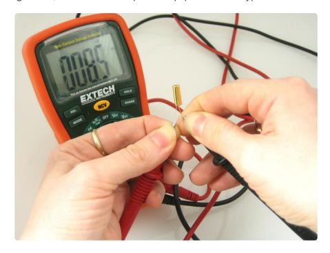
When pointing up, the switch is closed (low resistance / continuous).
