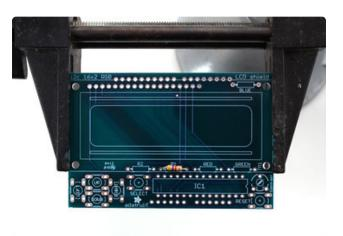
We'll start with the first resistor **R1** - which has yellow, violet, red, gold bands on it. This resistor is part of the interface between the Arduino and the 'port expander' that controls the LCD.
