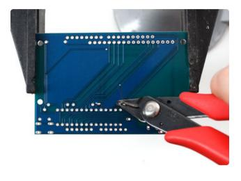
Once the soldering is complete, we can clean up by clipping the leads of the resistor. This keeps them from shorting to something else. Use diagonal or flush cutters to clip the wires right above where the solder joint ends.
