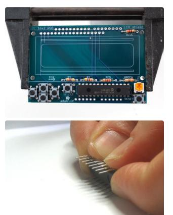
We're nearly done! Now we will place the I2C port expander chip. Double check that it has the MCP23017-E/SP marking on it. This is a 16-pin expander chip, that uses the i2c bus. That means you can send it commands using the i2c pins on an Arduino and control 16 more digital pins! 5 of those pins go to the buttons, 6 go to the LCD control and 3 are used for the backlight (the remaining 2 are unused).
