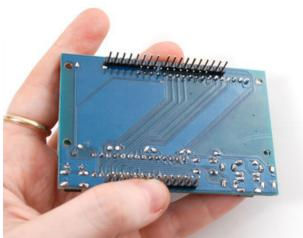
Finish up by carefully clipping the leads. For some Arduinos, the long leads may interfere with headers or parts on the Arduino board so we suggest just clipping them all. Do it carefully as these are a little difficult to cut and may fly at you. We suggest doing it over a trash can.
