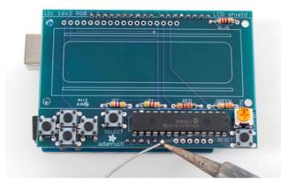
Solder all of the header pins. Even though they aren't used for passing signals, they will make the mechanical connection to the Arduino strong.
