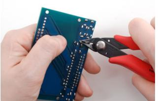
To make it sit flat, you may need to clip the legs of the buttons down - they will interfere with the DC jack, lifting the shield a bit.
