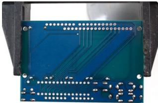
Solder each leg, taking care not to accidentally 'short' two button legs together. The ones for the directional pads are very close!
