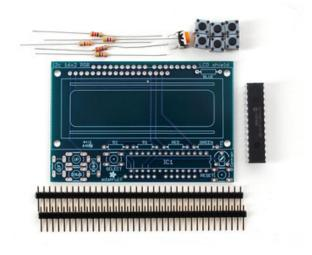
Check the kit against the <u>parts list</u> (https://adafru.it/cl9) to verify you have all the parts necessary
