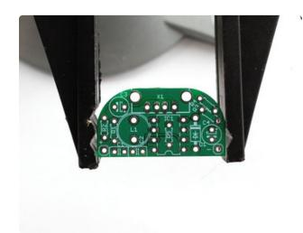
Place the PCB in a vise, and turn on the soldering iron. Make sure you have all the tools you'll need to assemble the kit (https://adafru.it/c3s).
