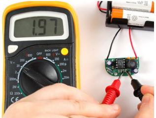
Next check between the rightmost pin and the second and third pin. They should both be at just about 2.0V
