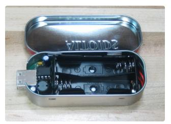
Once you're happy, remove the electronics and put the doublesided sticky foamtape on both the circuit board and the battery holder.
