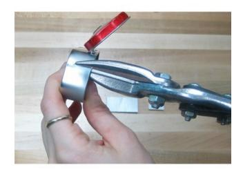
Cut two notches in the end of the tin, just about where the flat part ends and the tin starts to round out.
