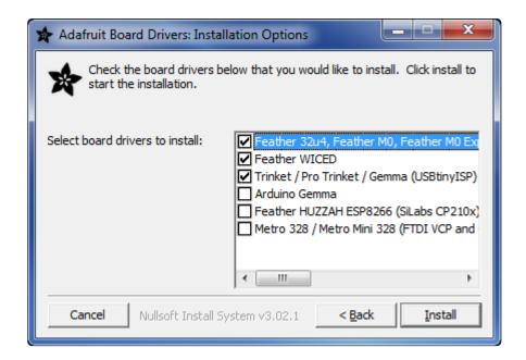
Once the installation process is complete, you should be able to plug your WICED Feather into your system and it will be recognized thanks to the signed drivers you just installed.
