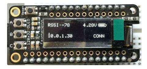
The data rendered on the display will depend on the way that you configure the example sketch, but the top and bottom lines are reserved for WiFi and LIPO information, and the two middle lines (referred to as the 'Message Area' in Adafruit\_FeatherOLED) can be used to render any text or messages.
