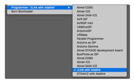
You can then click the **Burn Bootloader** menu entry and the Arduino IDE will attempt to use the JLink or STLink (via <u>AdaLink</u> (https://adafru.it/fPq)) to reflash the bootloader for you.
