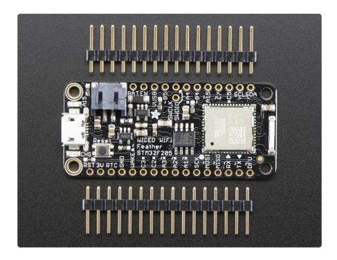
Comes fully assembled and tested, with a USB bootloader that lets you quickly use it with the Arduino IDE. We also toss in some headers so you can solder it in and plug into a solderless breadboard. Lipoly battery (https://adafru.it/e0v) and MicroUSB cable (https://adafru.it/aM5) not included (but we do have lots of options in the shop if you'd like!)
