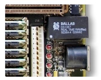
The image above shows a computer motherboard with a Real Time Clock called the  $\underline{D}$  S1387 (https://adafru.it/aX0). There's a lithium battery in there which is why it's so big.
