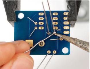
To keep the battery holder from falling out, you may want to 'tack' solder it from the top.
