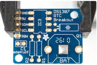
Begin by soldering a small bump onto the negative pad of the battery: this will make better contact!
