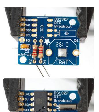
Place the two 2.2K resistors, and the ceramic capacitor. They are symmetric so no need to worry about direction. If you're planning on using with a Raspberry Pi (which has 3.3V logic and built in pull-ups, skip the 2.2K resistors!
