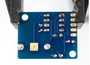
Clip the leads of the resistors, crystal and capacitor short.
