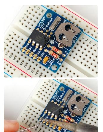
If you'd like to use the header to plug the breakout board into something, place the header in a breadboard, long side down and place the board so that the short pins stick thru the pads.
