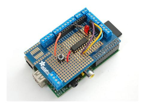
Now that you've finally got your hands on a Raspberry Pi® (https://adafru.it/aHx), you're probably itching to make some fun embedded computer projects with it. What you need is an add on prototyping Pi Plate from Adafruit, which can snap onto the Pi main board assembly (and is removable later if you wish) and gives you all sorts of prototyping goodness to make building on top of the Pi super easy.
