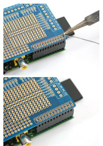
Heat up the soldering iron to 650 °F and wait for it to get up to temperature. Then heat a corner pad/pin with the iron tip and after two seconds poke in a small amount of solder. After the solder has melted into the pad/pin remove the iron.
