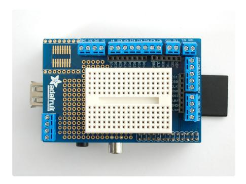
We designed the plates so you can fit a 'tiny breadboard' (http://adafru.it/65) on top and still see the pin labels on the breakouts. This makes it easy to do fast prototyping!
