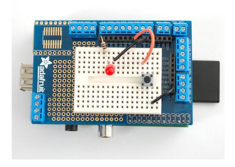
For more permanent projects, you can just place parts in and solder directly into the proto plate
