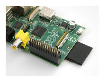
Place the big 2x13 pin header onto the Raspberry Pi GPIO breakouts so that it covers every pin. The connector is symmetric so it will fit on either way.
