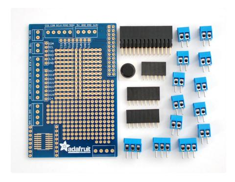
The layout of the board is a mix between 'breadboard style' (top middle) - with two 'rails' down the center and then 5-pin connected rows along-side. This layout is familiar for anyone who has used a breadboard. The remaining holes are 'perf' style - no connection between them. This allows for more flexibility.
