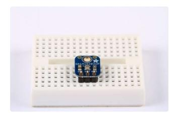
Position the breakout board Line the board up with the header pins and drop it in place for soldering.
