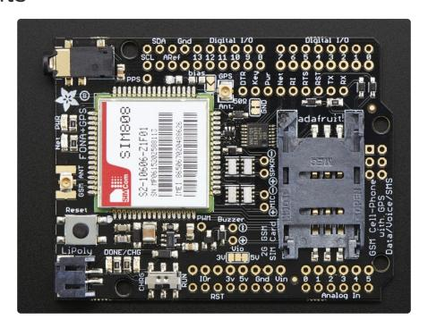
There's a lot going on in this shield, we basically stuffed an entire phone in here! So lets go piece by piece on what you get in a shield
