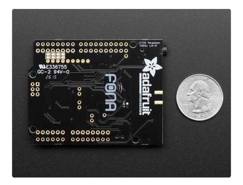
Each order comes with one tested and assembled FONA shield and a stick of 0.1" male header. Required Arduino, SIM card, battery, antenna and other accessories are not included! Some light soldering is required to put the headers onto the shield. You can also grab some stacking headers if you would like to stack a shield on top (http://adafru.it/85)
