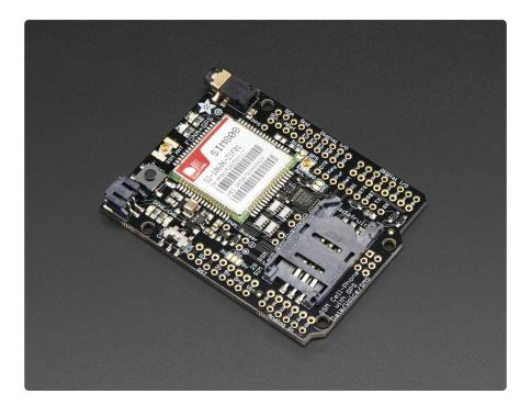
Cellular + GPS tracking, all in one, for your Arduino? Oh yes! Introducing Adafruit FONA 808 GSM + GPS Shield, an all-in-one cellular phone module with that lets you add location-tracking, voice, text, SMS and data to your project, in Arduino shield format for easy use.
