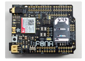
The SIM should be secure and flat in the holder
