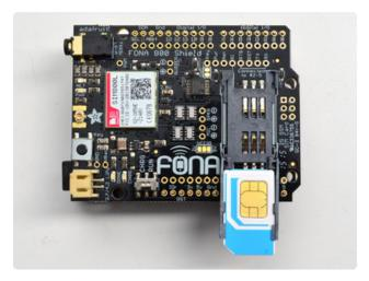
Insert the SIM with the gold pads facing up and the notch on the outer corner
