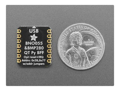
This PCB is designed to fit onto the back of any QT Py or Xiao board. It can be soldered into place or made removable using pin and socket headers.
