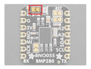
Address jumper - The I2C address changing jumper for the BMP280 is located to the left of the sensor (outlined in red in the board image). This jumper is open/not connected by default. If you solder the jumper closed, it will change the BMP280 I2C address from **0x77** to **0x76**.
