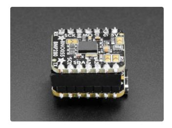
Connect the QT Py RP2040 with plug headers into the BNO055 + BMP280 BFF with socket headers. They should be plugged in with the backs of the boards facing each other.
