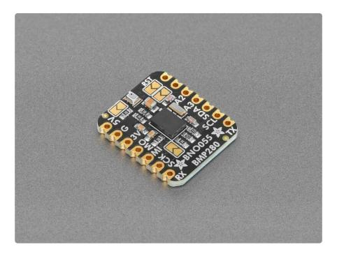
If you'd like, you can solder the BFF directly on the back of your Xiao/QT Py or use the included header to solder each side to your QT Py to make a sandwich. You can also pick up an Itsy Bitsy short female header kit to make it removable but compact (http://adafru.it/4174); you'll need to trim the headers to 7 pins long.
