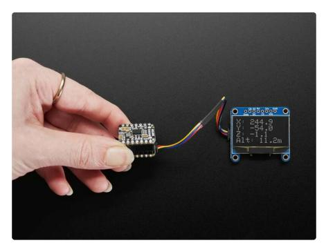
Usage for the BFF is simple because both the BNO and BMP talk over I2C - so you'll just use the SDA/SCL pins. Note that some QT Py boards with a Stemma QT port have two I2C ports, so make sure you are using the port that's on the SDA/SCL pins, not the QT port!
