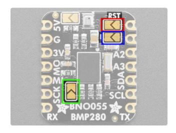
**RST** - The reset pin for the BNO055 is located next to pin **AO** (outlined in red in the board image). This jumper is open/not connected by default. If you solder the jumper closed, it will connect the reset pin to **AO**.
