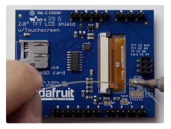
Next, apply a little solder to create a solder bridge on all three of the ICSP pads.
