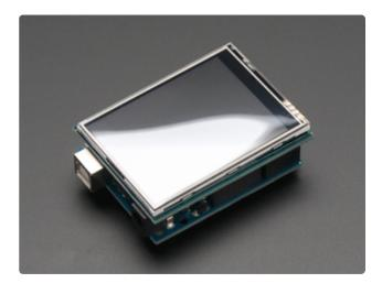
Plug the shield into your Arduino or Megashaped board. The GPIO pins are keyed and should only plug in one way.
