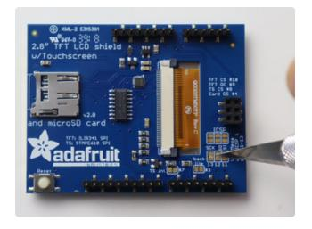
First start by taking a sharp knife and cutting the traces that connect to pins 11-13.
