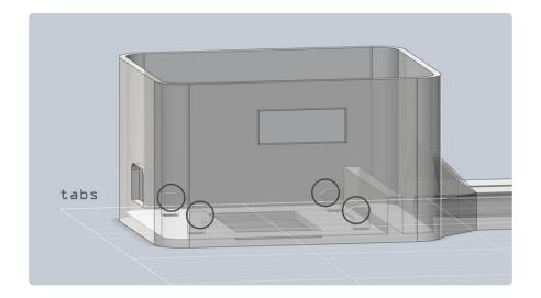
The **box.stl** part houses the 500mAh lipo battery and Trinket. At the bottom of the enclosure, the opening with tabs allows the **connector.stl** part to mount to the **hotshot.stl** part to the enclosure.
