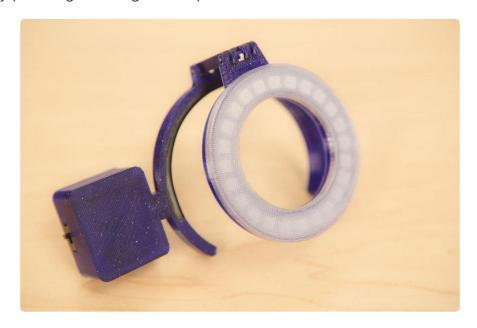
Close up the enclosure by snapping the lid on and slide the switch on to power up the ring! The clip snaps onto most DLSR camera lenses such as the 100mm or 24-70mm prime lenses.
