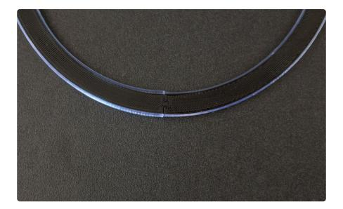
The neoring-60-top.stl and neoring-60-bottom.stl parts are the two pieces that snap together to make the large ring. The neoring-60-cap-top.stl and neoring-60-cap-bottom.stl parts are also two parts that snap together, these are to be printed in transparent PLA to diffuse the LEDs.
