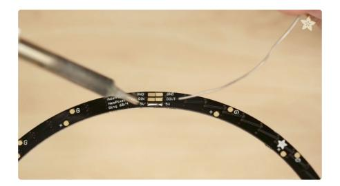
Start by soldering just two pieces together. Once you've aligned them up, apply a line of solder from one connection to there other. Make two sets of halves and solder those together.
