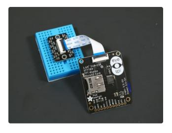
Repeat this process for the FPC connector on your display. Again, ensure that the **blue stripe** on either end of the cable is facing up.
