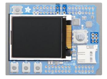
In the center is the 1.8" TFT display. This display is full color (16-bit RGB), 128x160 pixels, and has a backlight. The display receives data over SPI plus two pins:
