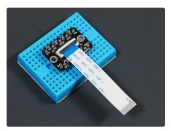
To secure the cable, lower the FPC connector latch onto the EYESPI cable.
