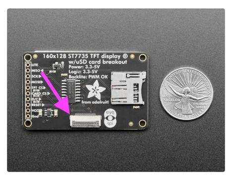
The EYESPI cables are 18 pin 0.5mm pitch flex cables. They are ~9.6mm wide, and designed to fit perfectly into the EYESPI connector. Adafruit currently offers EYESPI cables in three different lengths: 50mm (http://adafru.it/5462), 100mm (http://adafru.it/5239), and 200mm (http://adafru.it/5240).
