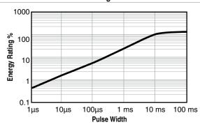
Although Ohmite's TFSS Series resistors have been specially designed and developed to absorb much more energy than standard resistors, pulses and transients require special consideration since they cause an instantaneous temperature rise in the resistor film. This application note can guide you through these considerations.
