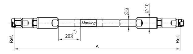
All dimensions are in mm; tolerances:  $\pm$  3mm for A  $\leq$  300 mm;  $\pm$  1% for A > 300 mm \*) If length "A" < 150 mm marking is mount centric  $\pm$ 5 mm
