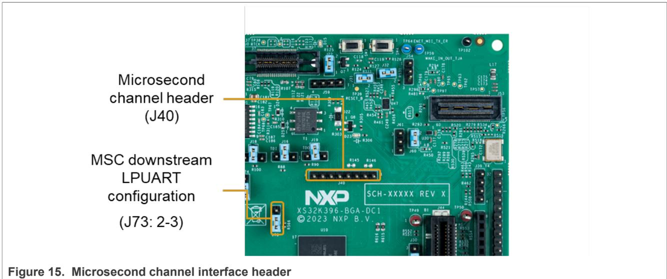
Figure 15. Microsecond channel interface header
