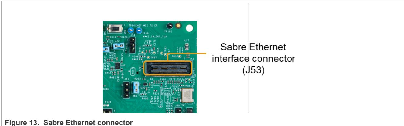
Figure 13. Sabre Ethernet connector
