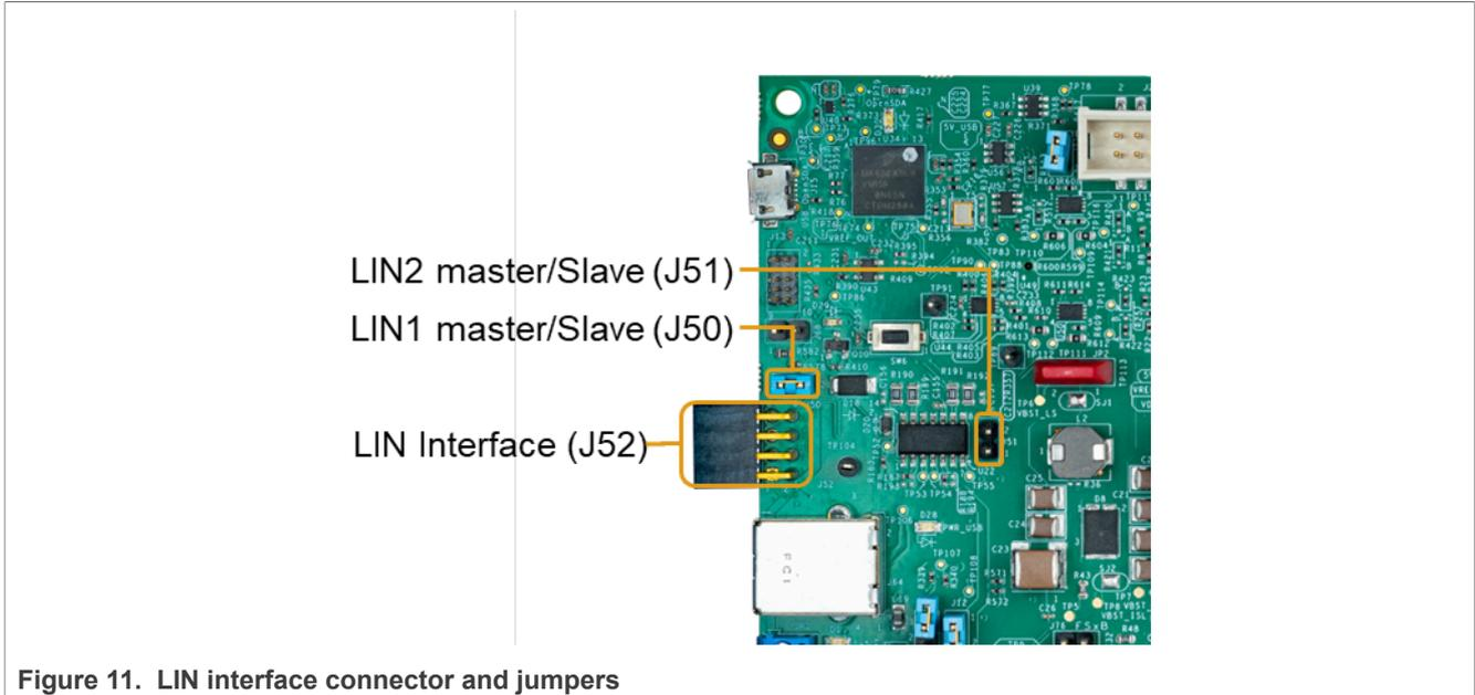
Figure 11. LIN interface connector and jumpers
