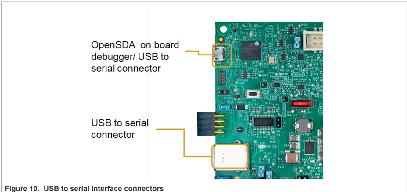
Figure 10. USB to serial interface connectors
