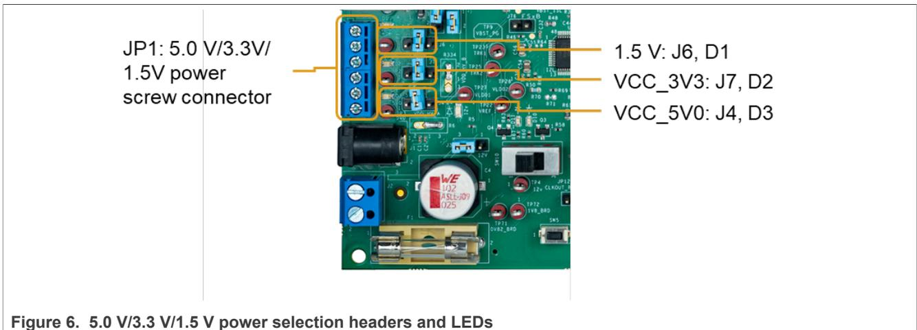
Figure 6. 5.0 V/3.3 V/1.5 V power selection headers and LEDs
