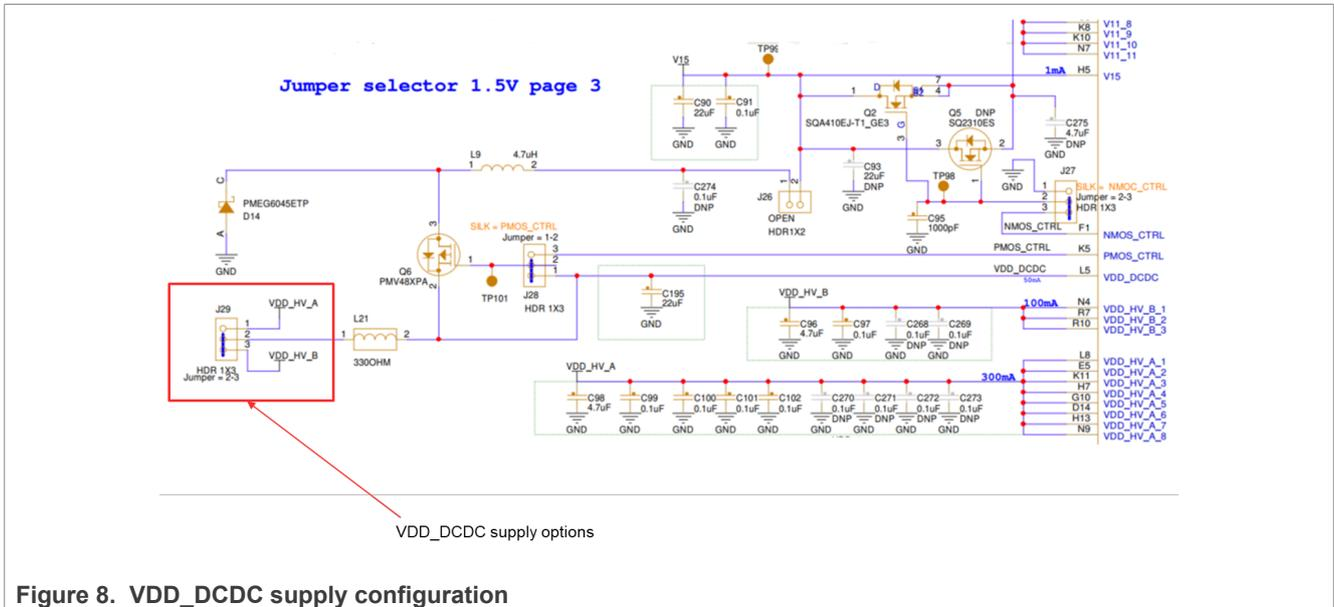
Figure 8. VDD\_DCDC supply configuration
