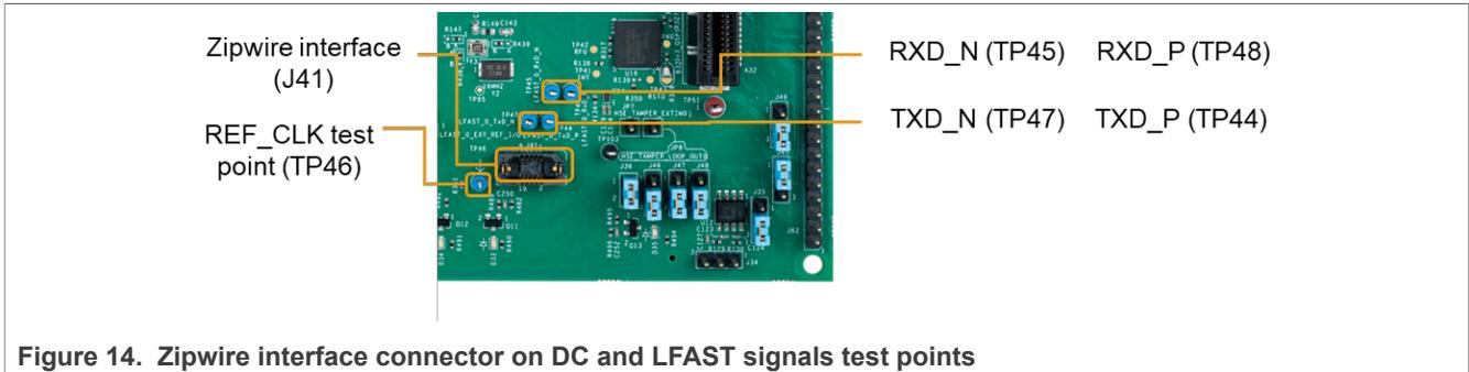
Figure 14. Zipwire interface connector on DC and LFAST signals test points
