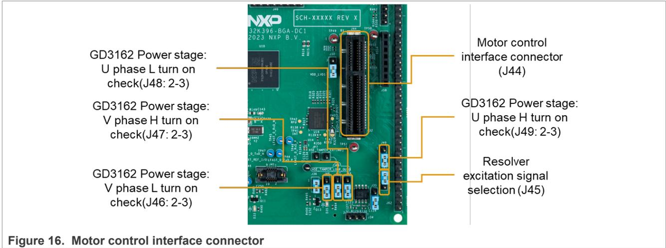
Figure 16. Motor control interface connector
