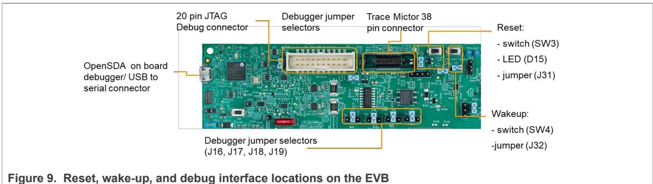
Figure 9. Reset, wake-up, and debug interface locations on the EVB
