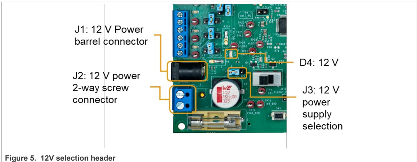
VCC\_12V is further used to supply VBAT\_LIN and as a supply for Ethernet PHY Sabre board that can be connected through connector J53.
