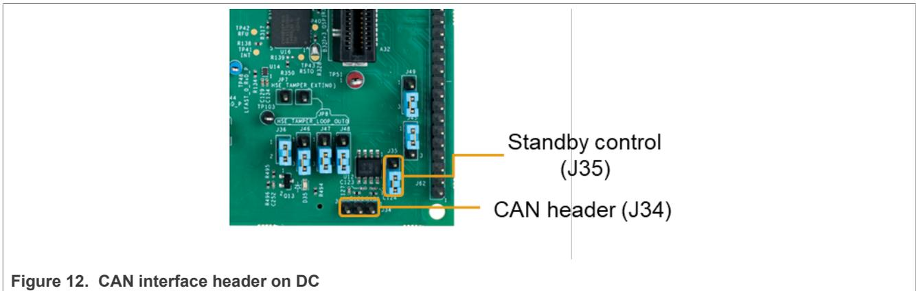
Figure 12. CAN interface header on DC
