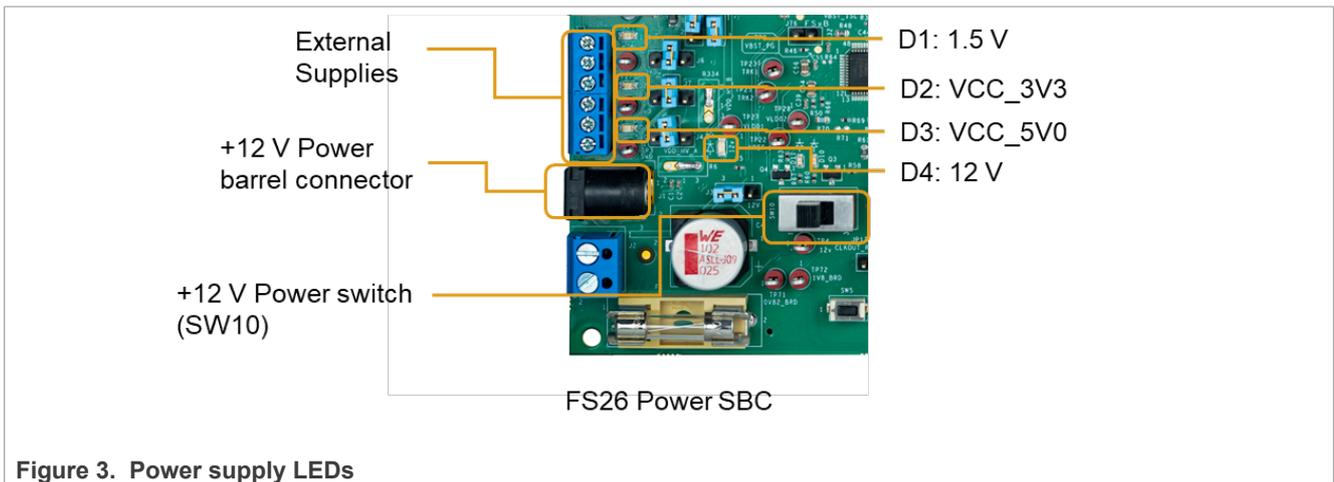
Figure 3. Power supply LEDs
