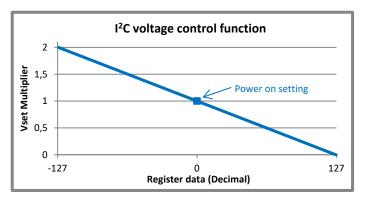
Example 1: OP1, Vset = 5V, Vadjust = 2V,  $I^2C$  address = 20h, Voltage adjust register = F8h
