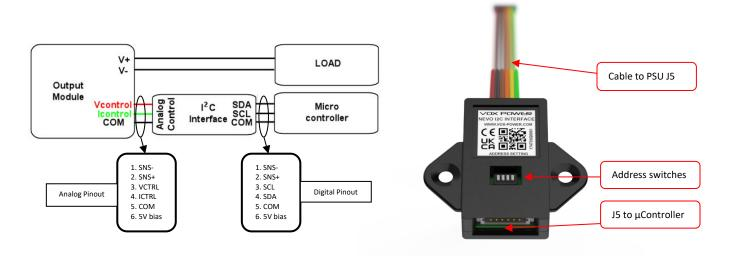
The output voltage and current limit can then be controlled in +/-127 steps that are programmed through the  $I^2C$  interface. Careful consideration must be given to system grounding as the interface is <u>not</u> isolated and must be referenced to the COM pin on J5. Incorrect system grounding may cause damage to the unit. Adhere to the same precautions as for "Local bias supply" detailed on page 16 of the user manual or contact Vox Power for assistance.
