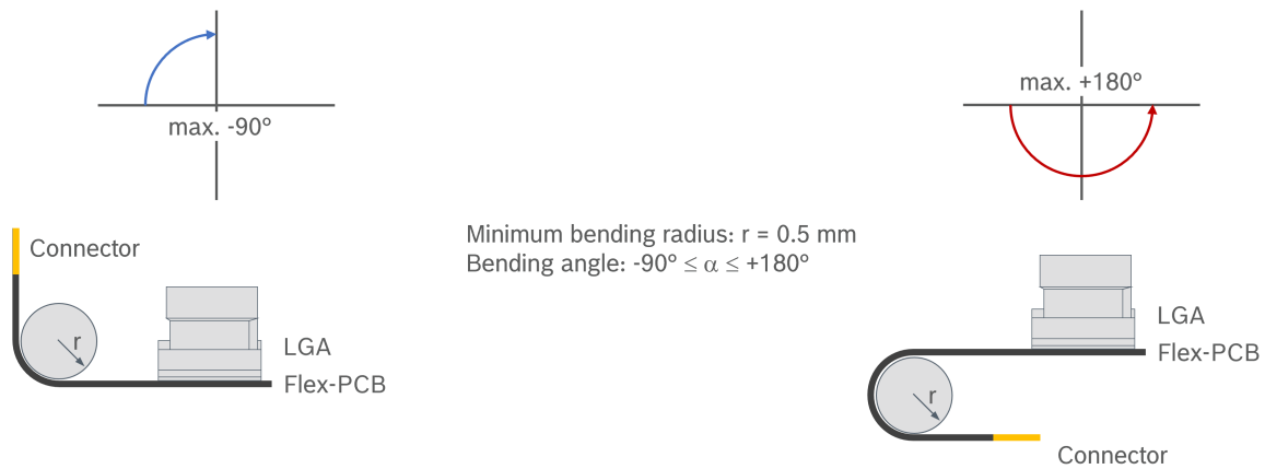
Figure 9: Maximum bending angles and minimum bending radius
