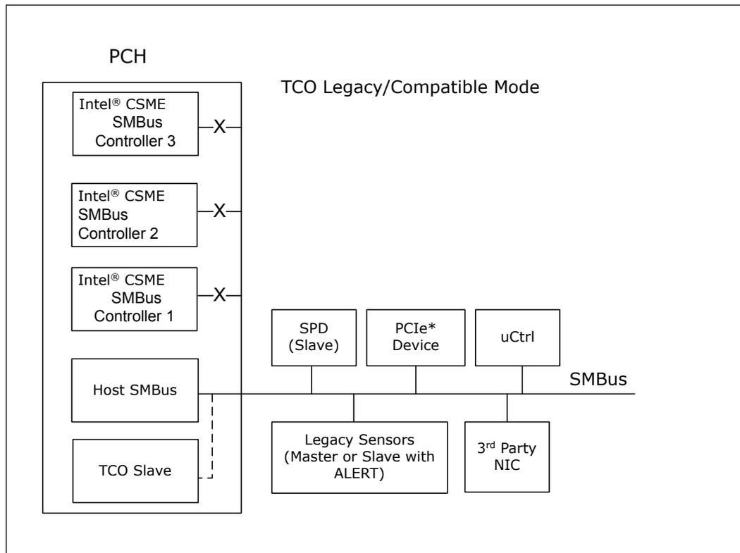
In TCO Legacy/Compatible mode the PCH can function directly with an external LAN controller or equivalent external LAN controller to report messages to a network management console without the aid of the system processor. This is crucial in cases
